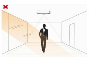
• Make sure there are no moving objects interfering in the counting area. For example, do not install the sensor too close to a door.
