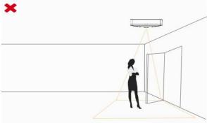
• Avoid installing the sensor near a mirror or avoid drawing the line to the mirror.
