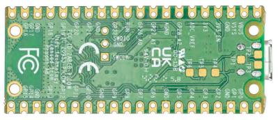
Raspberry Pi Pico W has been designed to be a low cost yet flexible development platform for RP2040, with a 2.4GHz wireless interface and the following key features:
