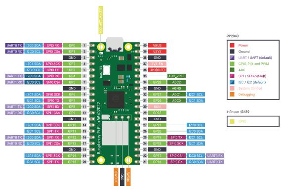
Raspberry Pi Pico W uses an on-board buck-boost SMPS which is able to generate the required 3.3V (to power RP2040 and external circuitry) from a wide range of input voltages (~1.8 to 5.5V). This allows significant flexibility in powering the unit from various sources, such as a single lithium-ion cell, or three AA cells in series. Battery chargers can also be very easily integrated with the Pico W powerchain.
